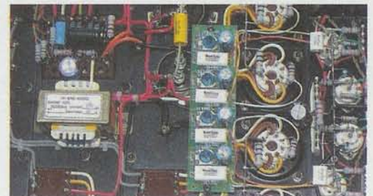
The unmodified inside of the ProLogue One.
