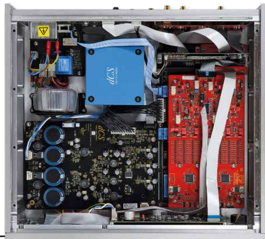
RIGHT: A Rossini PSU [brown PCB, lower left] is fed from a screened transformer [blue box] with the Vivaldi-inspired Ring DAC adjacent [red PCB]. The extra transformer [top left] feeds the optional headphone amp [lower right, on fascia]
