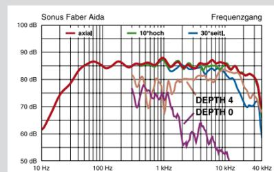
Despite the long chassis-to-chassis distances and the 3.5-way design, the Sonus Faber proves to be perfectly neutral with a wide dispersion angle. With "Depth" on 0, the loudspeaker radiates very low levels backward above 1.5kHz, with full depth the directivity index decreases to about 3-4 decibels.
