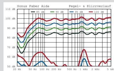
Very low distortion and clean, impressive reserves notably in the bass range. The tiny distortion peak around 1 kHz is due to a resonance, but inaudible. With 109 decibels the Aida has also a very high power handling, the more so as it can unleash still greater reserves in the sub and kick bass range.
