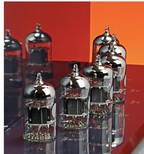
*A rank of 12AU7 double triode small signal valves handle preamplification (2) and phase splitting/buffering (4).*
