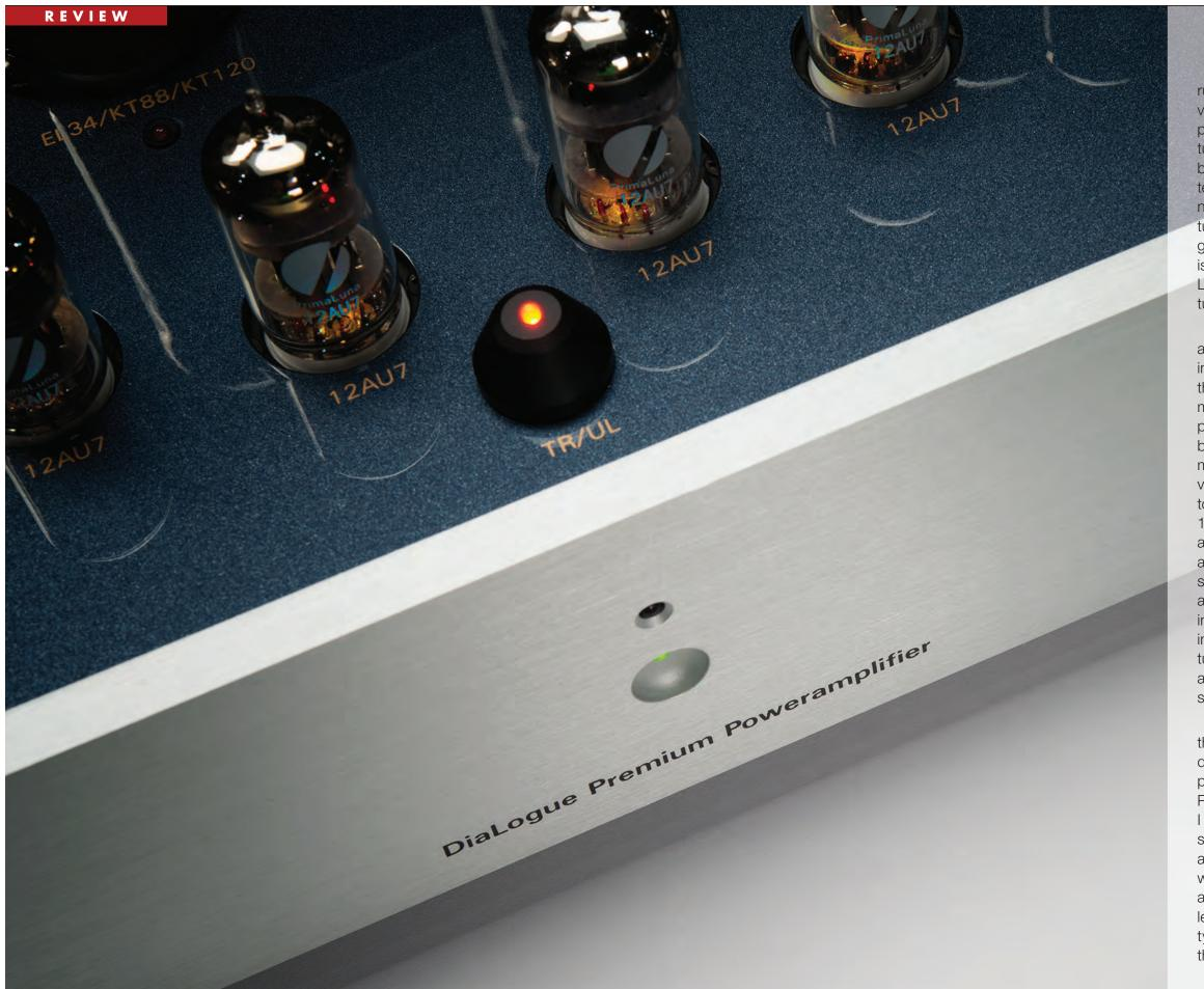
Fortunately, the DiaLogue Premium runs the output tubes very conservatively, and thanks to PrimaLuna's patented Adaptive Auto Bias, adjusting tube bias is a thing of the past. The benefits are multiple: Tube life is extended, distortion is reduced, and the need for a matched quartet of output tubes is eliminated. It's as painless as it gets for a vacuum-tube amplifier. There is even a Bad Tube Indicator, a red LED that lights up, should an output tube fail.
