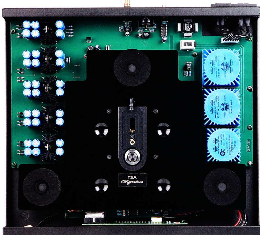
**RIGHT:** Metronome employs a Philips CDM12 Pro 2 disc mechanism, modified in-house. Power supply has three transformers separately feeding critical parts of the transport
