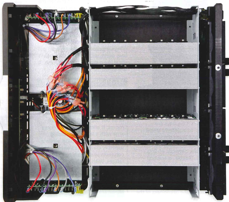
RIGHT: A dual-mono amp in a single chassis with two separately screened power supplies and no fewer than eight pairs of Motorola PowerBase 100W output transistors per side
