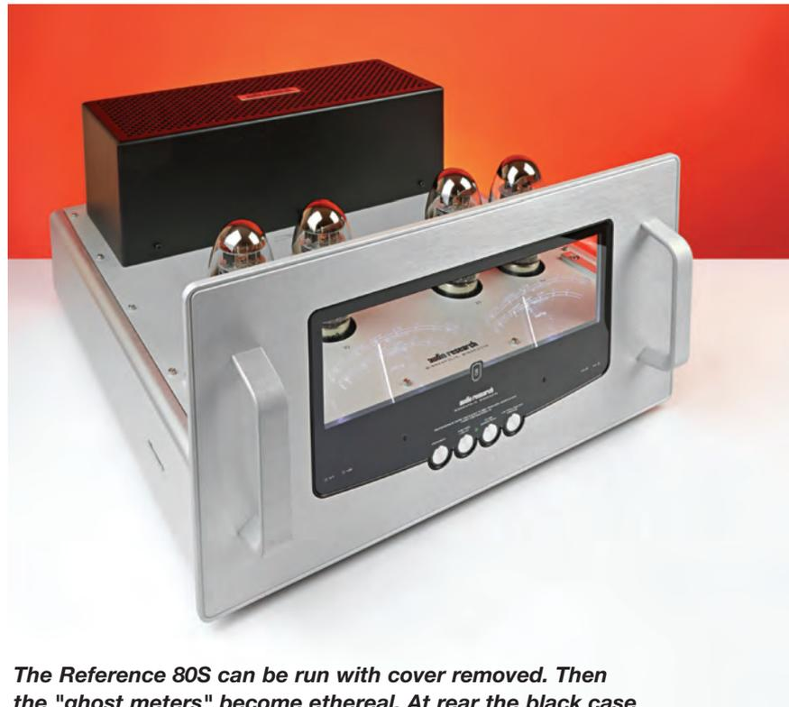
**The Reference 80S can be run with cover removed. Then the "ghost meters" become ethereal. At rear the black case screens mains and output transformers.**
