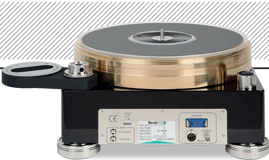
**ABOVE:** As with all TechDAS decks, pneumatic hoses from an outboard pump [see below] are connected to air-bearing 'Flotation' and LP hold-down 'Vacuum' fittings while power, pump and speed controls are communicated via a multi-pin connector
