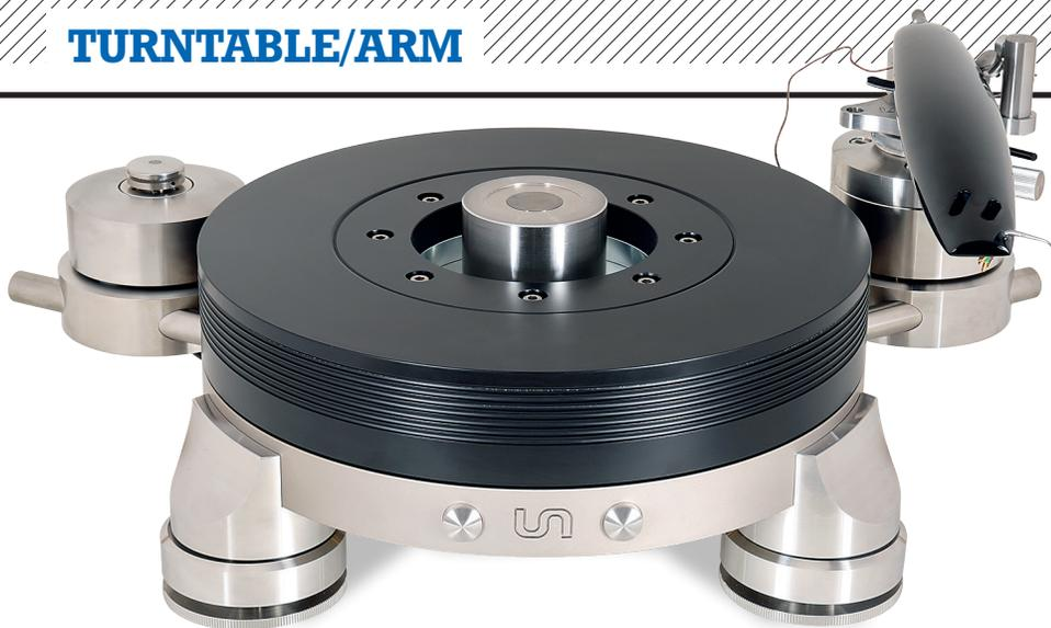
**ABOVE:** With uppermost platter removed, the black Delrin/alloy 'mid-platter' is revealed in position over the massive stainless steel/tungsten bearing. Grooves accept the round-section drive belt
