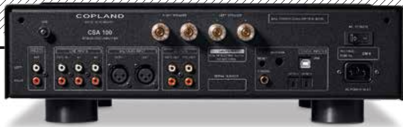
ABOVE: MM phono is joined by a tape loop, three line ins (two on RCAs, balanced on XLRs), a preamp out and single sets of 4mm speaker terminals. Digital inputs include coaxial, two optical and USB. Note hole for forthcoming Wi-Fi/BT streaming adapter
