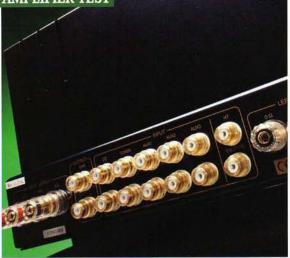
ABOVE: On the rear of the amp can be found five line-ins, a tape loop, a home theatre input that bypasses the preamp section, plus 4 and 80hm speaker taps
