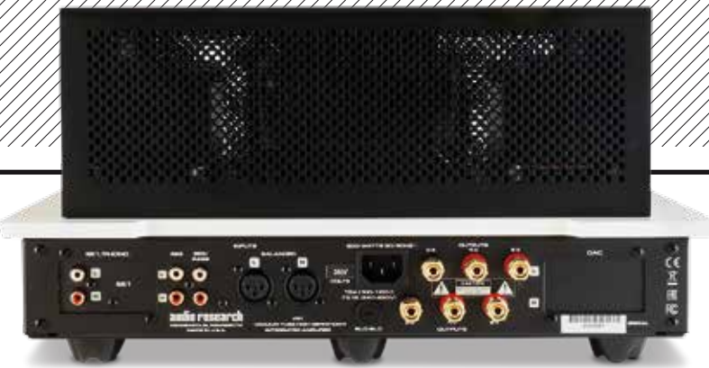
ABOVE: Three single-ended line ins on RCAs (one pass through) and a balanced set on XLRs are joined by 8 and 4ohm speaker taps on gold-plated 4mm binding posts. Note spaces that will accommodate the phono [left] and DAC [right] modules
