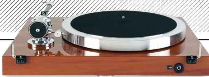
ABOVE: The C-Note arm's counterweight is damped by a sorbothane-like polymer while the nylon thread for the bias outrigger sits in a groove around the arm base, improving stability. The tonearm leads connect via a five-pin SME/DIN connector
