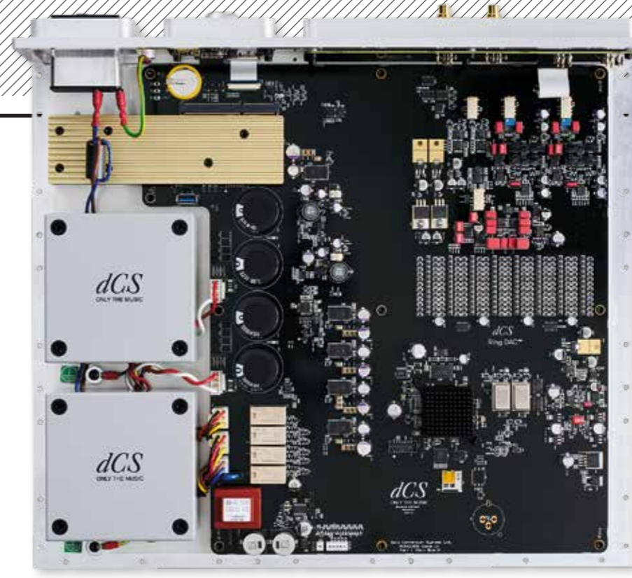
LEFT: Inside the Varèse Mono DAC with dual PSUs [left] powering the Xilinx DSP [heatsink], Ring DAC's differential matrix of 2x48 resistor current sources [centre right], and mixed op-amp based analogue output stage [top right]
