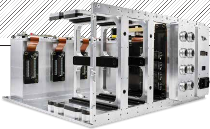
ABOVE: Inside the machined alloy case of the Varèse Core showing the (screened) main PSU and USB-A/Ethernet digital inputs [far right] with ruggedised bays [near left] waiting for the optional digital I/O expansion modules to be fitted
