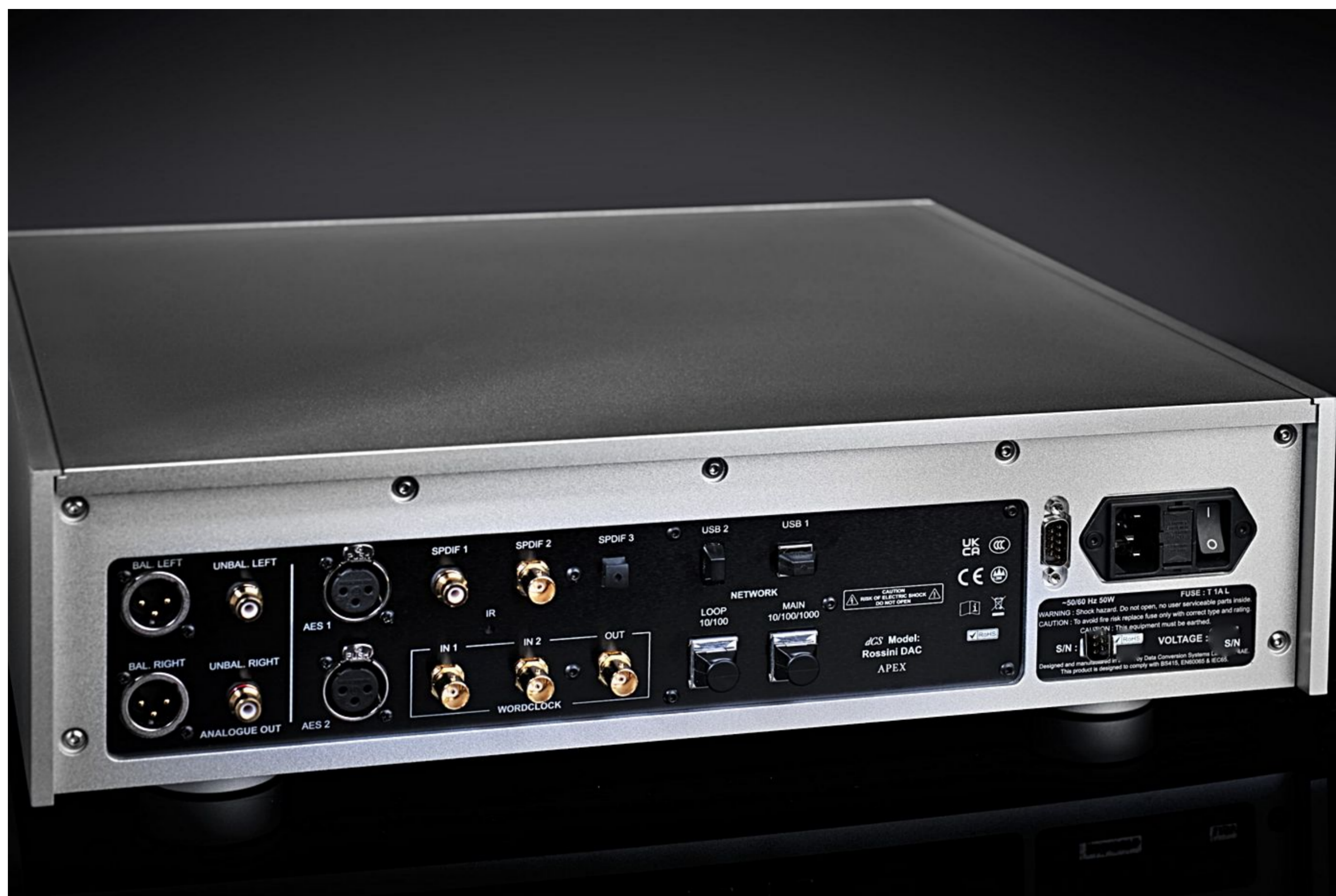
At the back, balanced and single-ended outputs; inputs 2 x AES/EBU on XLR, 1 x BNC, 1 x SPDIF on RCA and optical Toslink, USB A and B. Plus BNC in and out connectors for an external clock. (photo courtesy dCS)
