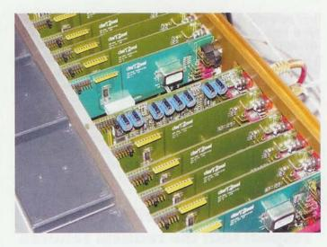
input to accept an umbilical from the outboard charger, along with earth tags for the phono section, toggles to apply 6dB of attenuation on certain inputs, and other toggles to defeat ABOVE: To reduce signal degradation through switches and relays, each source input is a pre-amp in its own right BELOW: Space for missing badge on pre-amp awaits personalised plaque
