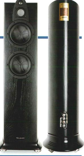
Wharfedale's claim of 87dB sensitivity for the Jade 5 looks a little optimistic given our measured pink noise figure of 85.8dB, while the nominal impedance of 60hm is given a minimum modulus of 2.7ohm. Poorly controlled impedance phase angle results in the EPDR dipping to a minimum of 1.2ohm at 73Hz – a pretty scary figure for a speaker in this price range.
