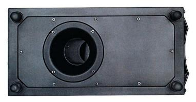
A large port fires downwards toward the floor. This loads the rear drive unit and has an output that reaches right down to produce subsonics. The feet have rubber pads that conceal spikes that can be used as an option.
