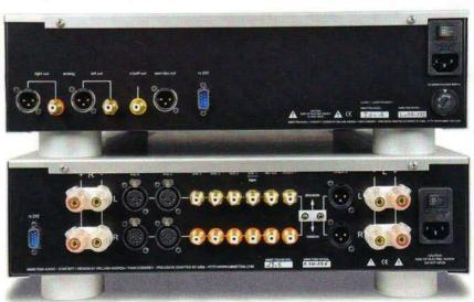
In RCA phono and XLR form that can be used in absolute and relative modes - the former being full signal for a recorder and the latter being variable for a subwoofer or second power amplifier. As the weight suggests, construction is on the solid side, with a 10mm aluminium front plate, 10/15mm 'processed iron' chassis and a 10/15mm aluminium top plate, with damping to minimise resonance.
