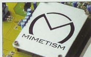
Metal plate covers upsampling and digital-to-analogue converter
