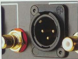
Player offers both single-ended and XLR balanced outputs to the rear
