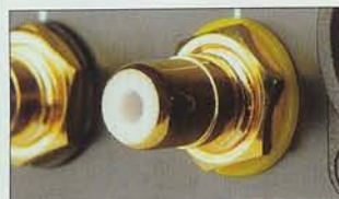
S/PDIF output on a sturdy RCA, and isolated from the digital power supply
