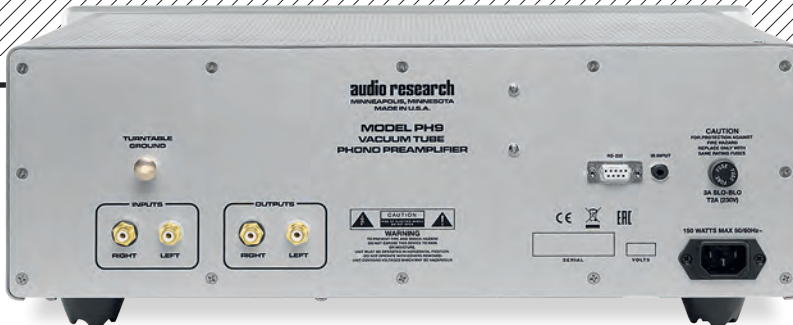
ABOVE: Could not be simpler – a single set of RCA phono inputs (with ground post) and another pair of RCAs for the RIAA-equalised output. RS232 services automation
