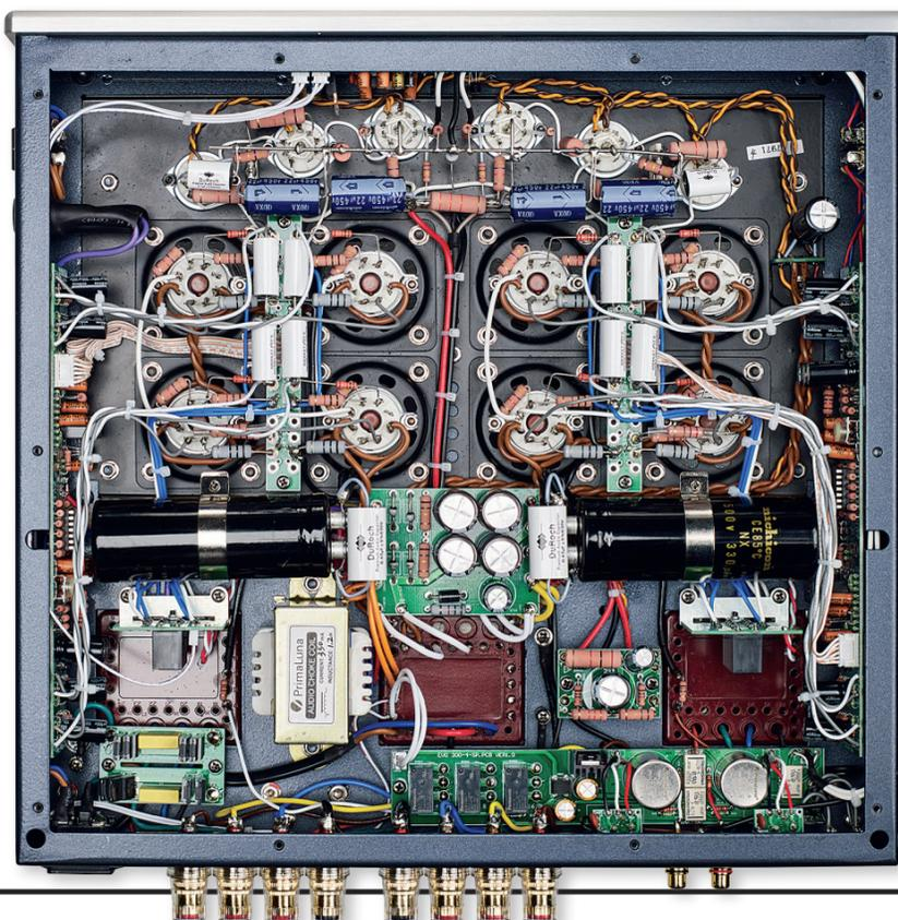
**RIGHT:** Underneath the EVO 400 power amp reveals its dual-mono construction with high quality tube bases [top], point-to-point wiring with Teflon insulation, and choke-regulated PSU with tube rectification [lower left]
