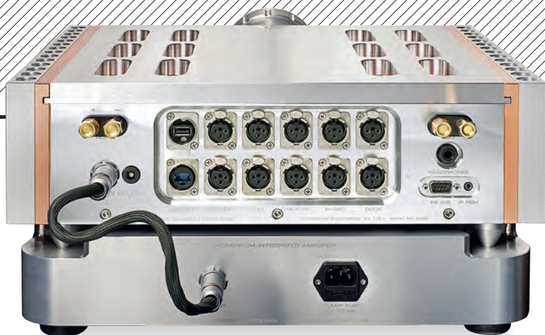
ABOVE: Fed via a short umbilical from its outboard DC PSU/isolation platform, the MLife offers five balanced inputs plus USB, Toslink and networked digital audio (via an external router). Pairs of speaker binding posts and a headphone out are included
