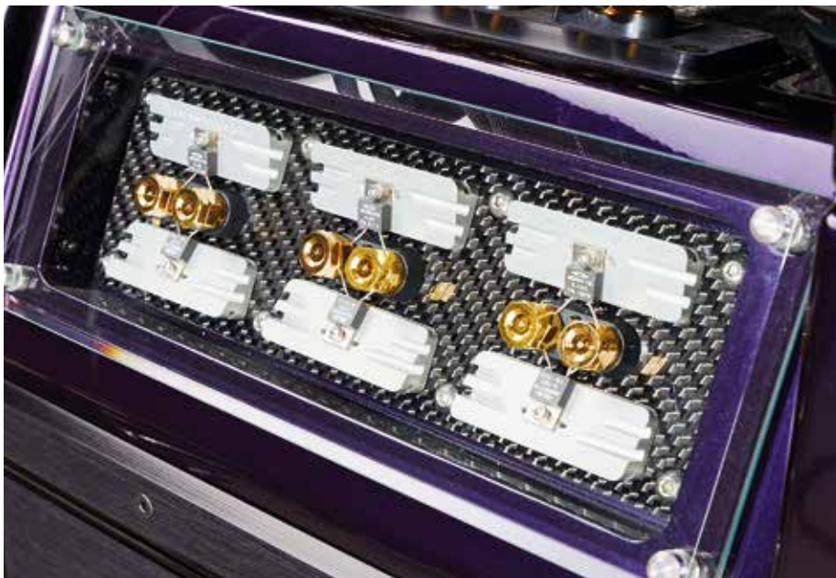
ABOVE: Rear-mounted protection and tuning resistors for the mid and treble drivers are now illuminated, for easy access and visibility. The high-pass mid/treble crossover is also mounted inside the upper section of the bass cabinet
