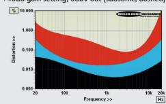
ABOVE: Distortion vs. frequency (20Hz-20kHz) at 100mV out (black), 500mV (blue) and 1V out (red)
