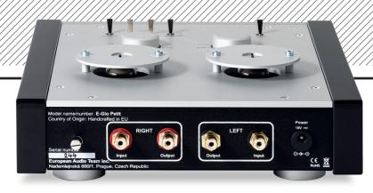
**ABOVE:** Simplicity itself – single gold-plated RCAs for connection to the tonearm leads and out to your choice of (pre) amplifier. Note  $\pm 18V$  DC PSU input socket
