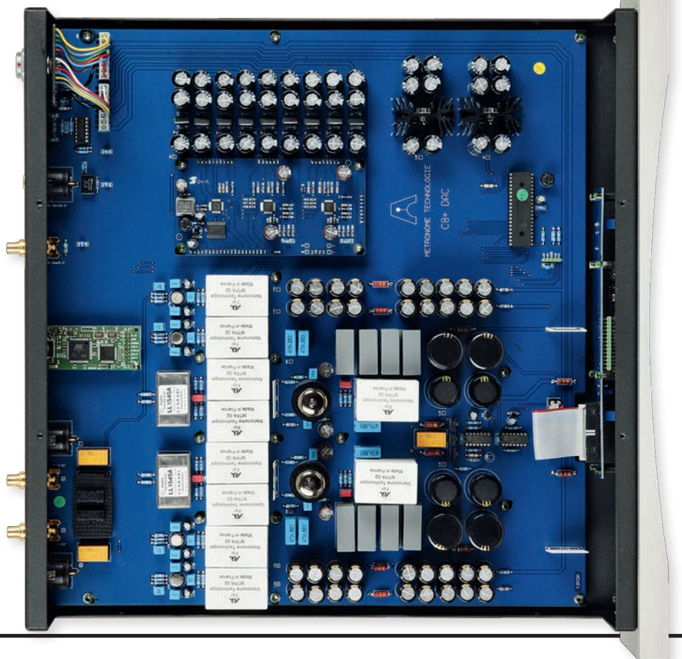
RIGHT: The C8+ is based around a pair of sophisticated 32-bit AK4490 DACs (resampled to 96kHz), features custom passive components and transformer-coupled balanced analogue output stages (solid-state and 6922 tube-based)
