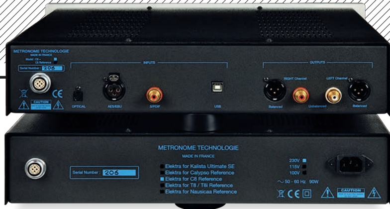
ABOVE: USB plus optical and coaxial S/PDIF and AES/EBU digital inputs with balanced (XLR) and single-ended (RCA) analogue outs. PSU connects via umbilical
