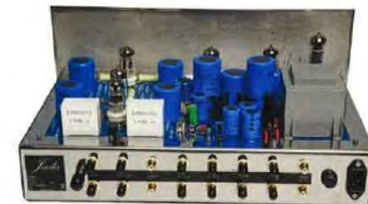
**Once the protection cage has been taken off, we have access to all the components of the preamplifier which includes the two power supply regulation tubes, the four double triodes, all the capacitors and resistors.**
