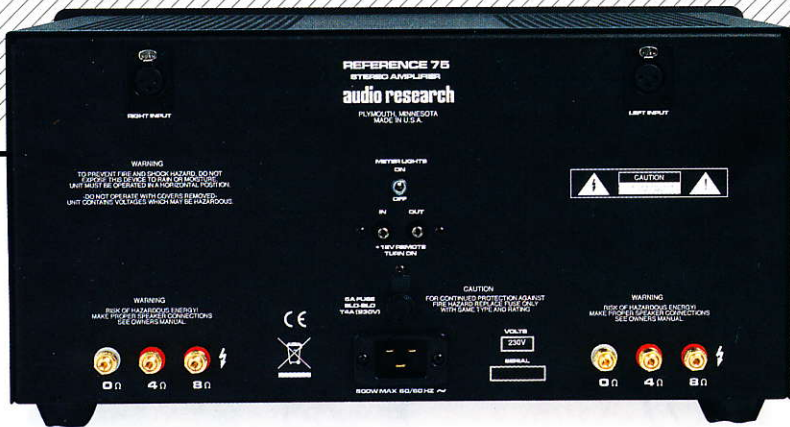
ABOVE: Meter illumination is switched on/off here. Balanced (XLR) inputs only plus screw-down 8ohm and 4ohm speaker terminals. These will accept bare wire and are sufficiently well-spaced to accommodate 4mm spade adapters
