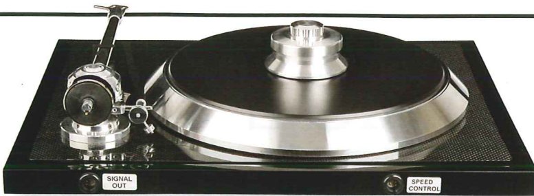
ABOVE: The C-Note arm's counterweight is damped by a sorbothane-like polymer while the nylon thread for the bias outrigger sits in a groove around the arm base, improving stability. The arm/signal out and PSU sockets use colour-coded connectors
