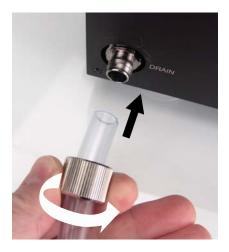
To drain, push the included PVC tubing onto the barbed fitting marked "Drain" and screw on the knurled compression ring. Position the opposite end of this tubing into a sink or large container to capture the older water.
