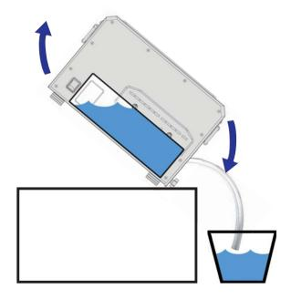
Once the reservoir is completely empty, unscrew the rear access cap. If the unit will be shipped or transported, paper towels can be placed inside the reservoir to absorb residual water (along with replacing the access cap).
