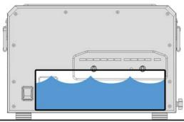
Keep unit level whenever water is inside. Always drain water from the reservoir completely before transporting.
