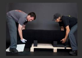
With two people, lift the speaker from the bottom and move the speaker down on the base of the crate until the top of the speaker is lying in the middle foam rib of the crate.
