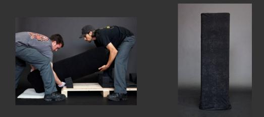
Tilt Speaker up on to a soft surface, Make sure that back of speaker does not hit the crate and that the binding posts do not touch the floor.
