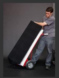
If it is necessary to move the speaker from the crate to the listening position, use a hand truck with a study piece of foam to protect the speaker.
