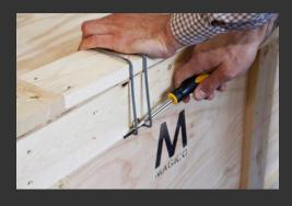
Remove 10 clamps using a flat-head screwdriver or pry bar.
