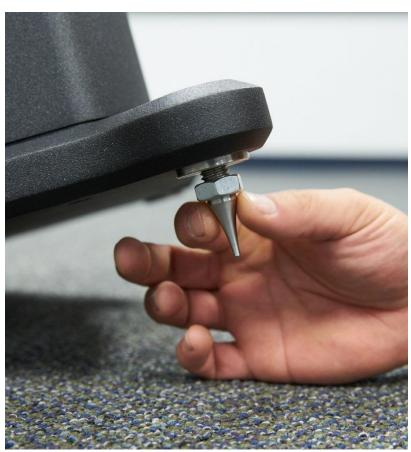
**15.** (OPTIONAL: FOR USERS WITH HARDWOOD FLOORS / TWO PEOPLE REQUIRED) WITH THE SPIKED SPEAKER SITTING FIRMLY ON THE FLOOR, ONE PERSON (STANDING) TO ONE SIDE SHOULD LEAN THE SPEAKER TOWARD THEM ONLY ENOUGH TO ALLOW THE SECOND PERSON (KNEELING) TO SLIDE A FLOOR SAVER DISC UNDERNEATH BOTH LIFTED SPIKES AND ALIGN THE SPIKE TIPS INTO THE CENTER HOLE OF EACH FLOOR SAVER DISC.
