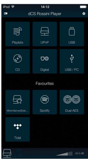
Tap UPnP to select a NAS on the same network. (Alternatively, tap USB/iPod to select a flash drive connected to the USB2 port.)
