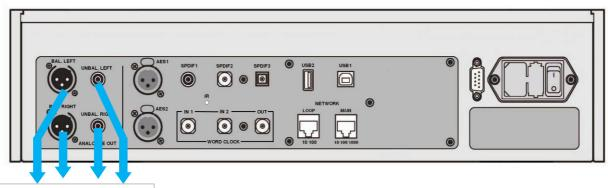
Balanced or unbalanced Analogue outputs to pre- or power amplifier
