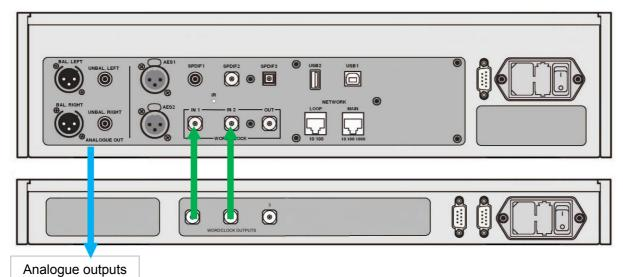
Figure 5 – Using the Rossini DAC and Clock together
