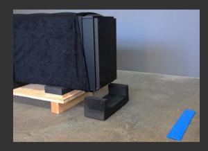
PLACE 'C'-SHAPED PIECE OF FOAM UNDERNEATH BOTTOM EDGE OF SPEAKER, SO THAT IT WILL FALL INTO THE MIDDLE OF THE FOAM WHEN TILTED UPWARD. IF UNPACKING ON A HARD SURFACE, PLACE SOMETHING SOFT WHERE THE FRONT OF THE SPEAKER WILL ULTIMATELY TOUCH THE GROUND, ADJUST IT AS NECESSARY WHEN LOWERING THE FRONT EDGE TO THE GROUND.
