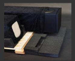
POSITION 2 PIECES OF FOAM FROM THE CRATE UNDERNEATH BOTTOM EDGE OF SPEAKER AS SHOWN IN THE PICTURE, SO THAT IT WHEN LIFTED UP, THE BINDING POSTS WILL HAVE CLEARANCE. IF UNPACKING ON A HARD SURFACE, PLACE SOMETHING SOFT WHERE THE FRONT OF THE SPEAKER WILL ULTIMATELY TOUCH THE GROUND, ADJUST IT AS NECESSARY WHEN LOWERING THE FRONT EDGE TO THE GROUND.
