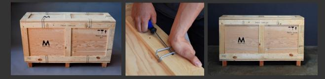
POSITION THE CRATE AS CLOSE AS POSSIBLE TO THE FINAL LISTENING POSITION. USING A FLAT HEAD SCREW DRIVER CAREFULLY REMOVE 10 METAL CLAMPS, HOLDING ONTO THE CLAMPS SO THAT THEY DO NOT FLY OFF.
