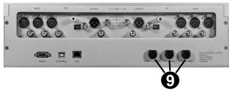
These inputs connect to the power outputs of the Perseus's separate power supply. The Perseus power supply includes permanently attached, spiral-wrapped, gold-plated copper cables designed for aerospace use. Each cable is rated to handle 30 amps.
