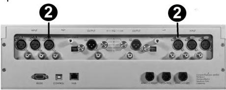
The two XLR inputs closest to the center of the Perseus back panel are for use with MM cartridges. As you are looking at the rear panel, the left XLR input is for the right channel, the right input is for the left channel. These XLR connections cannot be used concurrently with the RCA input below them; for example, you can use either MM-1 (XLR) or MM-2 (RCA), but not both. Use of XLR connections is
