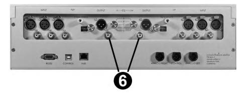
RCA unbalanced outputs are also supplied for preamplifers not equipped with XLR connections. When connecting to an amplifier, be sure to match the output to the correct channel on your amp. As you are looking at the back of the Perseus, the output on the left side is for the right channel, and the output on the right is for the left channel. To remove an RCA plug, grasp it by the connector body and pull the plug out.
