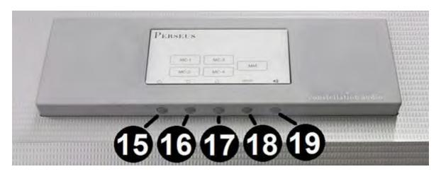
The front panel includes an LCD touchscreen and five buttons positioned underneath the display. These buttons work along with the touchscreen to provide control and monitoring of most Perseus functions. The functions of the buttons are shown using icons on the screen. Here are the functions:
