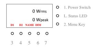
By pressing DIM key the display will dim off after 2 to 15 seconds (see chapter 10.1.). Pressing again will cancel the auto dimming function.
