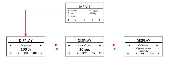
You can choose the illumination brightness. Press OK to confirm brightness setting, and then use the "+" and/or "-" keys to choose between 25, 50, 75 or 100%. Press OK again to memorize the brightness level.
