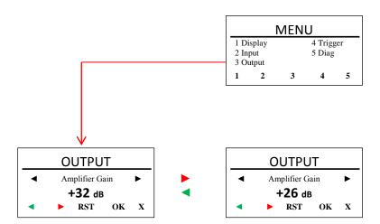
Here you can change the overall amplification gain. Press OK to confirm or use the arrows to select the desired gain, and press OK again for confirming the new setting. Factory default is 32 dB. Press X to exit the Output menu.
