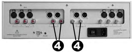
RCA unbalanced outputs are supplied for amps and recording devices not equipped with XLR inputs. The signal at these outputs is the same—it does not matter if you use output 1 or output 2.
