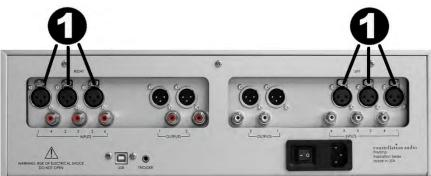
On the rear of the PREAMP 1.0 there are eight XLR inputs, four on each side. As you are looking at the rear panel, the left four XLR inputs are for the right channel, the right four inputs are for the left channel. Underneath each jack is the corresponding input number. Use of XLR connections is recommended for the best possible audio quality. To remove an XLR plug, push on the tab above the jack and pull the plug out.
