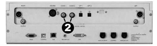
Use one of these connections if your digital source does not have AES/EBU. This connection is preferred to Toslink optical. The coaxial inputs accept PCM digital audio signals in resolution up to 32 bits/96 kilohertz. To remove an RCA plug, grasp the plug and pull it straight out. Do not pull on the cable.
