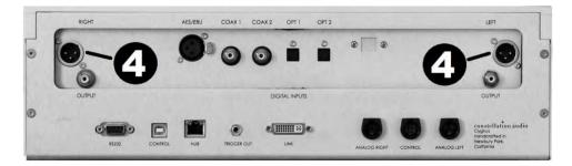
If your preamp or integrated amp has XLR inputs, use these outputs to connect the Cygnus, because they deliver the best sound. To remove an XLR plug, press the tab on the plug and pull the plug out.
