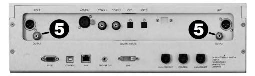
If your preamp or integrated amp does not have XLR inputs, use these RCA outputs to connect the Cygnus. To remove an RCA plug, grasp the plug and pull it straight out. Do not pull on the cable.
