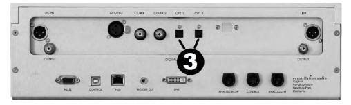
Use one of these connections if your digital source device does not have AES/EBU or coax. These inputs accept PCM digital audio signals in resolution up to 32 bits/96 kilohertz. To remove a Toslink connector, grasp the connector and pull it straight out. Do not pull on the cable.
