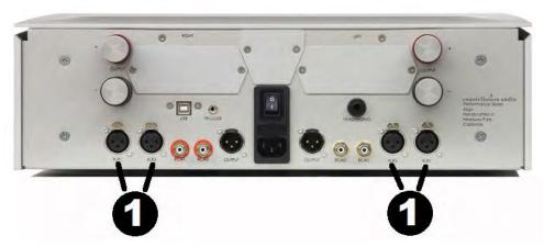
On the rear of the Argo integrated amp are four XLR inputs, two on each side. As you are looking at the rear panel, the left two XLR inputs are for the right channel, the right two inputs are for the left channel. Underneath each jack is the corresponding input number. Use of XLR connections is recommended for the best possible audio quality. To remove an XLR plug, push on the tab above the jack and pull the plug out.
