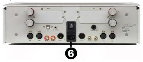
This connector accepts a standard 15-amp IEC AC connector. You can use the AC cord supplied with the Argo, or substitute your own cord. Before making this connection, turn the power switch above the AC input off. Connect the AC cord to the Argo, then plug the AC cord into the wall or your power conditioner, then turn the Argo's power switch on.
