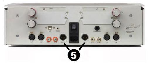
The two inner XLR connections on the rear of the Argo are outputs. These can be connected to a larger, more power amplifier such as the Constellation Audio Hercules or Centaur. They can also be connected to a system in a second room, or to a powered subwoofer.
