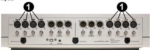
On the rear of the Altair II preamp there are eight XLR inputs, four on each side. As you are looking at the rear panel, the left four XLR inputs are for the right channel, the right four inputs are for the left channel. Underneath each jack is the corresponding input number. Use of XLR connections is recommended for the best possible audio quality. To remove an XLR plug, push on the tab above the jack and pull the plug out.
