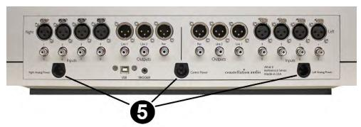
These inputs connect to the power outputs of the Altair II's separate power supply. The Altair II includes special spiral-wrapped, gold-plated copper cables designed for aerospace use. Each cable is rated to handle 30 amps.
