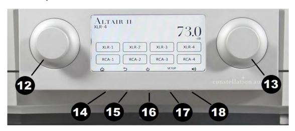
The front panel includes an LCD touchscreen and two knobs plus five buttons positioned underneath the display. These buttons allow you to control the Altair II without its remote. The functions of the buttons are shown using icons on the Here are the functions of the buttons and knobs:
