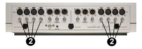
These unbalanced inputs are provided as a convenience for use with unbalanced signal sources. Whenever possible, we recommend using XLR connections instead. Connecting to an unbalanced source is handled in the same way an XLR balanced source.
