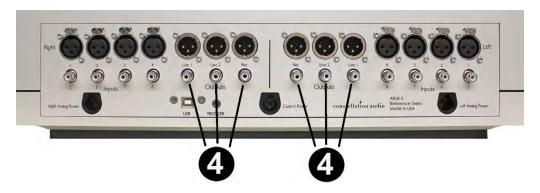
RCA unbalanced outputs are supplied for amps and recording devices not equipped with XLR inputs. The signal at these outputs is the same—it does not matter if you use output 1 or output 2.
