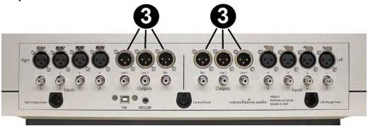
The inner six XLR connections on the rear of the Altair II are outputs. The signal at these outputs is the same—it does not matter if you use output 1 or output 2. To remove an XLR plug, push on the tab on the connector body and pull the plug out.
