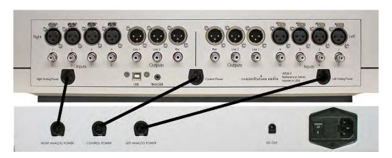
The Altair II's separate power supply (bottom component in the picture above) must be connected to the Altair II main chassis (top component in the picture above) as shown above before you plug the unit into a wall. Make sure the power switch on the power supply is in the off (O) position.
