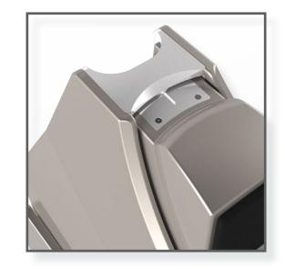
the tweeter module, the specific location of which determines the propagation delay position of the tweeter module within the Upper Array. The alignment plate contains numbered indents. The alignment tables in Section 6 contain the information for positioning the tweeter module in the array, determined by the indent in which the cross member's spike rests.
