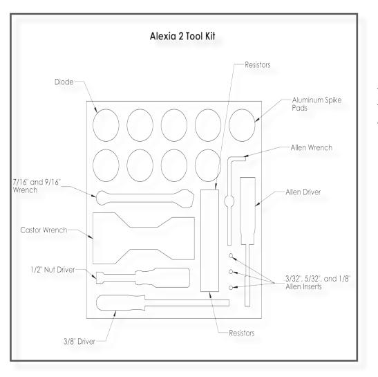
You will be using tools and parts in this kit throughout the installation process. Keep the Alexia Series 2 toolkit at hand.
