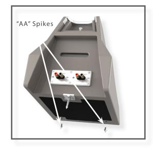
"AA" spikes are always installed in the front two positions (the threaded holes located near the bottom front of the enclosure). The spike-type is stamped in the round top of the spike. The two "AA" spikes screw into the Upper Array. The spikes should be screwed in all the way, until they are hand tight. Do not over tighten spikes.
