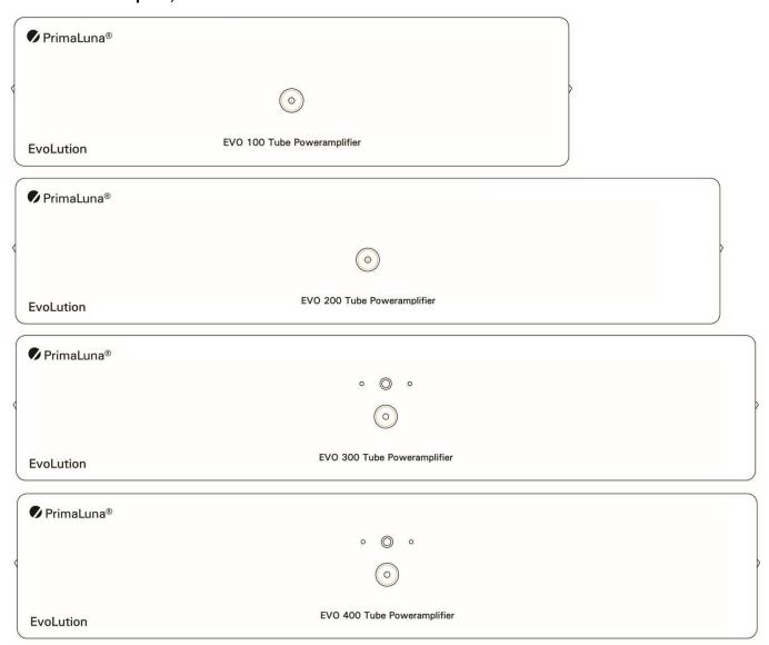
PrimaLuna front panels are made from machined aluminium, finished to match the black/blue metallic chassis. No controls are available from the front. The power switch and auto bias fuse are located on the left side of the amp, just behind the front plate, the bias switch on the right side, just behind the front plate.
