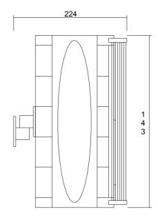
**SYSTEM**: 2 way vented box loudspeaker.
