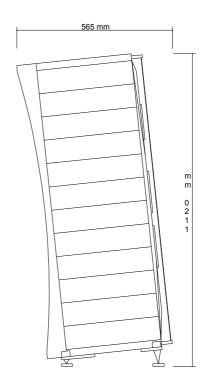
**SYSTEM**: 3 way floorstanding vented box loudspeaker.
