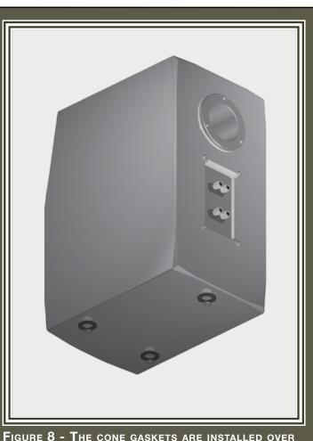
FIGURE 8 - THE CONE GASKETS ARE INSTALLED OVER THE GEOMETRIC CONES.
