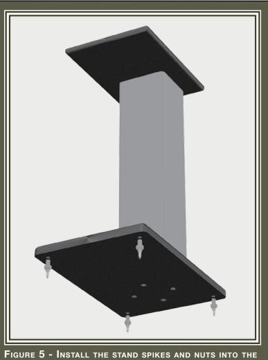
FIGURE 5 - INSTALL THE STAND SPIKES AND NUTS INTO THE THREADED HOLE ON THE BOTTOM OF THE STAND PLATE.
