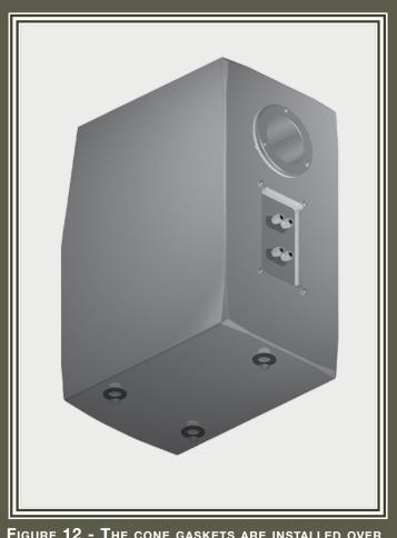
FIGURE 12 - THE CONE GASKETS ARE INSTALLED OVER THE GEOMETRIC CONES.
