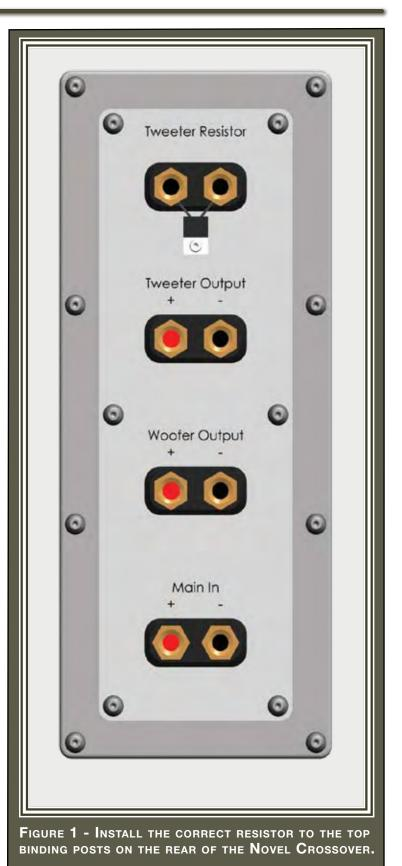
install the Allen screw so that the resistor is snug against the rear plate.
