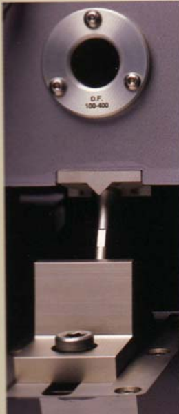
The upper module redesign adds a rear port, seen here above the 30 position Group Delay mechanism.
