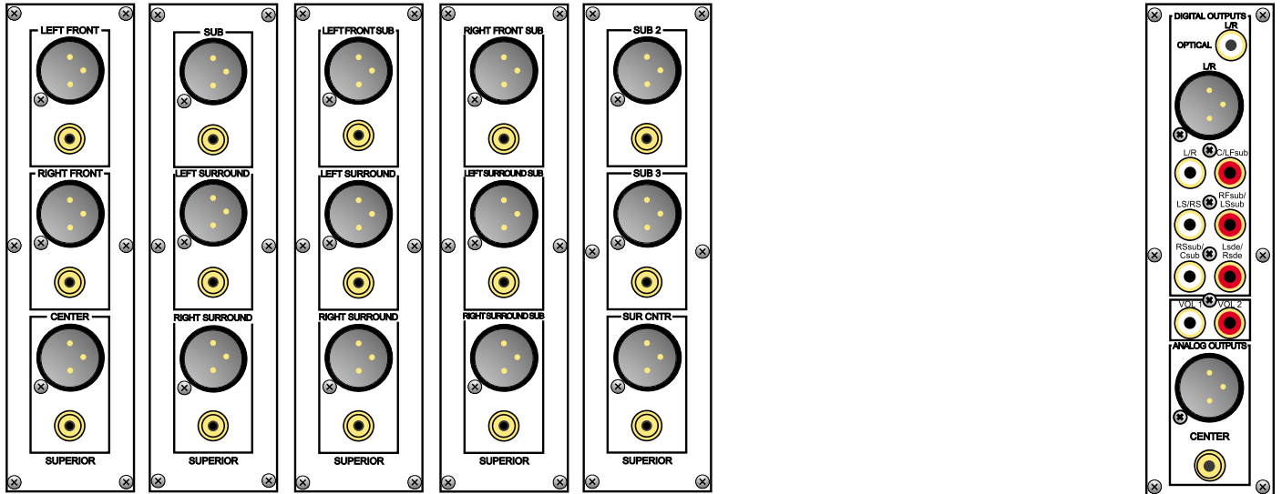
Figure 10 - All optional Superior D/A Cards and the Digital Output card with Center Channel
